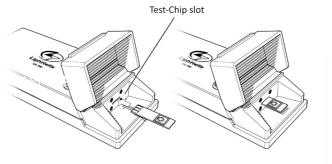
Side up the test-chip, plug into the testing slot
